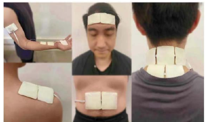
Figure 2: Modular design can be worn on different positions of the body.
